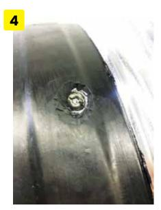
Remove the dowel until the nipple is exposed. Then replace the spoke or the nipple normally.
