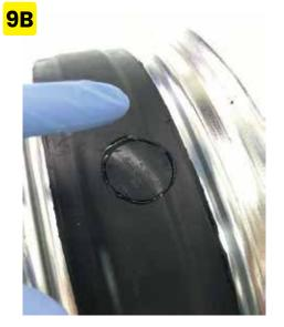
Wait a few hours: when the patch is no longer moveable to the touch, you can reassemble the tire carefully.
