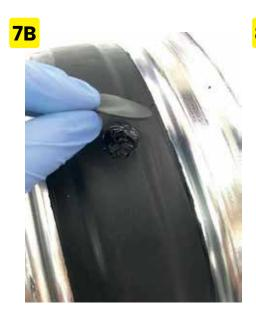
Apply the patch (included) directly on the fresh polymer before it hardens.
