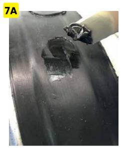
With a cutter blade or a spatula, level the polymer by removing the excess material.
