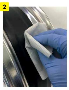
Carefully clean the surface to be treated with a common nitro paint diluent..
