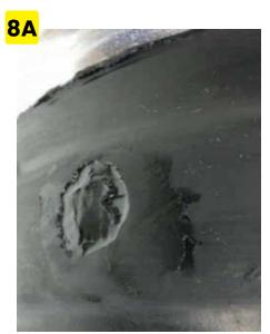
Wait 24-48 hours for the complete polymerization of the product before reassemble the tire.
