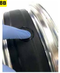
Firmly press until the excess material is overflowed, then remove excess.
