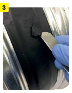
With the blade of a cutter, cut the polymer around the nipple until a dowel is obtained.
