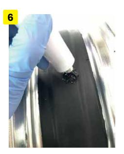
Apply an abundant amount of BARTubeless® polymer directly from the tube to the point to be repaired.
